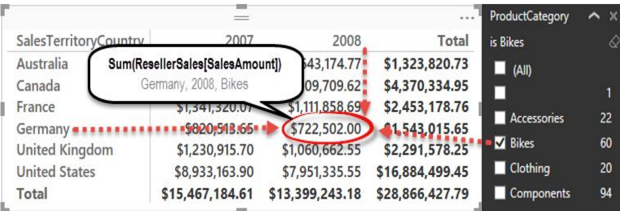
Figure 10.1 Measures are evaluated for each cell, and they operate in the cell filter context.
